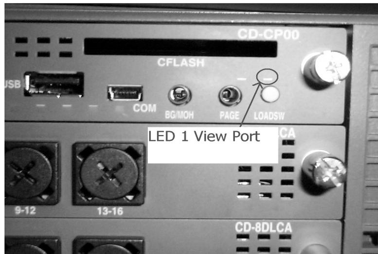
Figure 1-4 Checking LED1
